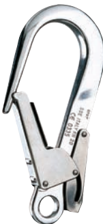
PETZL MGO Karabiner 460gm 60mm opening, with double safety system, for clipping to cables or metal rails.
